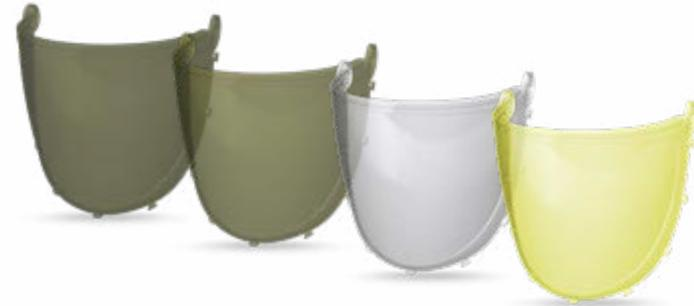
You can choose from two different shade levels 4 and 5 or a bright yellow visor. The brand new toric visors offer excellent optical quality (EN 166 class 1) and enhanced robustness - protection against high-speed particles with HIGH energy guaranteed and against molten metal and hot solids.
