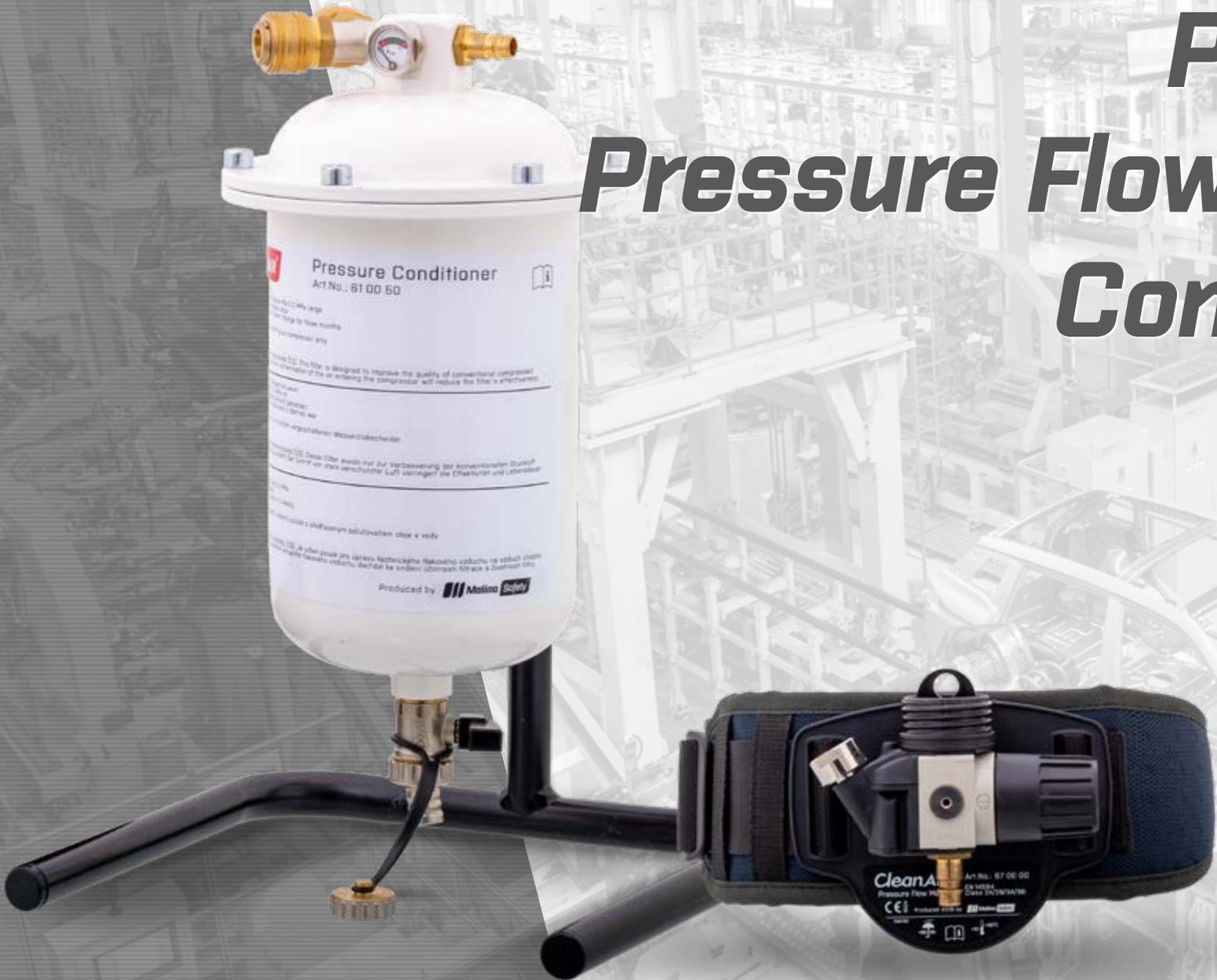
Systems CleanAIR® Pressure/Pressure Flow Master are constant flow supplied air respirators suitable for a long term work in the heaviest industrial environments. The regulator on the belt unit can adjust the amount of air coming from the central compressed air distribution system or a compressor and keeps it at a constant level without regard to the changes of inlet pressure.
