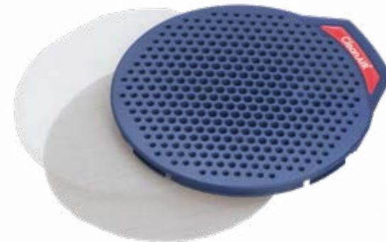
The spark arrestor prevents the filter from damage by hot sparks and spatters while the pre-filter traps the coarse particles and thus prolongs the lifetime of the main filter. Start using spark arrestors and keep your filter maintenance cost low.
